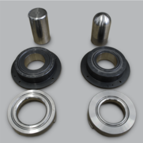
Tools for the forming limit curve (FLC) to ISO 12004
