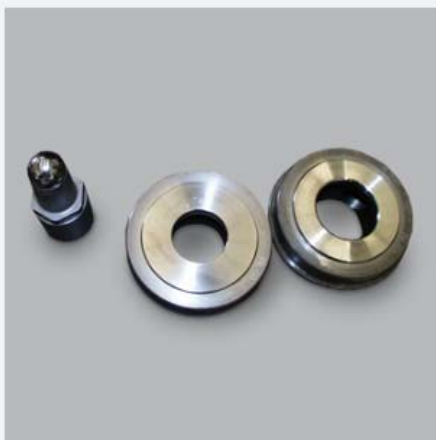
Tools for the cupping test to Erichsen or Olsen (ISO 20482 / ASTM E643-84)
